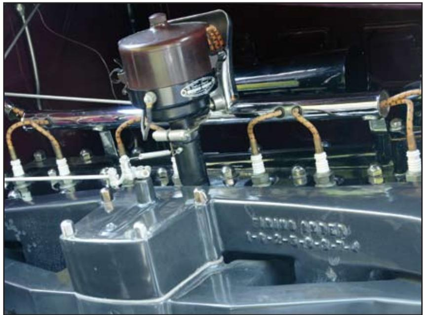
**CARBS:** Below these manifolds, the Pierce-Arrow carries a Stromberg "Duplex" carburetor with each of its two barrels feeding four cylinders. Pierce-Arrow's quality and attention to detail show in the construction of the ignition system. The distributor and ignition wire carriers did not need to look this nice to run well, but through touches like these, Pierce-Arrow made sure the customer knew he was getting what he paid for.
