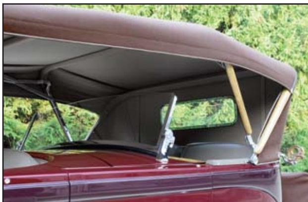
Usually, a four-door convertible without glass side windows is a touring car. With the addition of a second cowl and windshield for the rear seat, the car transforms into what Pierce-Arrow called a sport phaeton.
