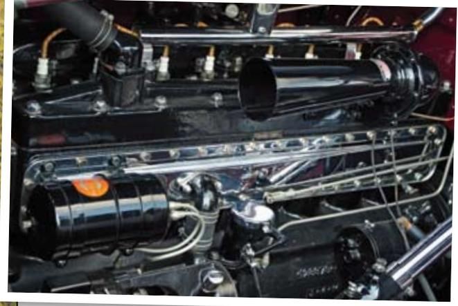
**ENGINE:** The Group B engine was Pierce-Arrow's middle-sized straight-eight in 1930. Its 366 cubic inches produced 125 horsepower. Technological advancements included a camshaft-driven fuel pump instead of a vacuum tank and a factory oil filter.
