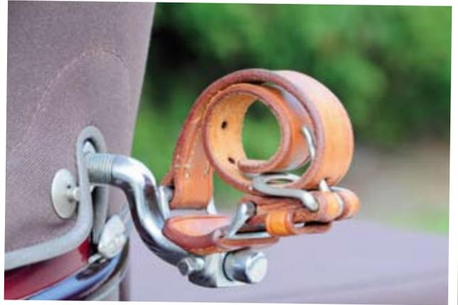
**DETAILS:** This Pierce-Arrow received a very detailed restoration. These leather straps hold the top and boot cover in place when the top is lowered.
